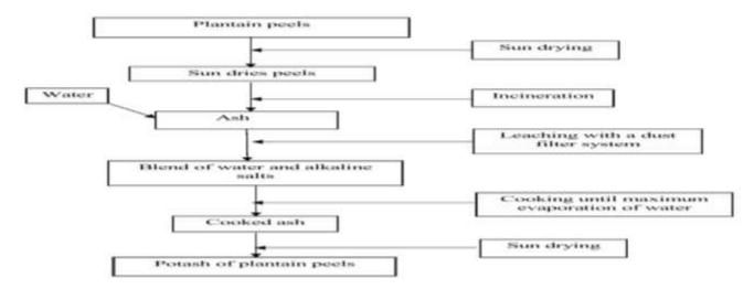
Figure1: Traditional plantain peels potash manufacturing diagram
